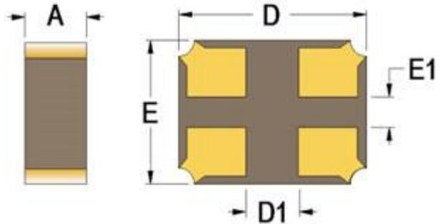
Here is the IPC-7351 calculated footprint, select the "Footprint" tab - Compared to the mfr. pattern (right)
